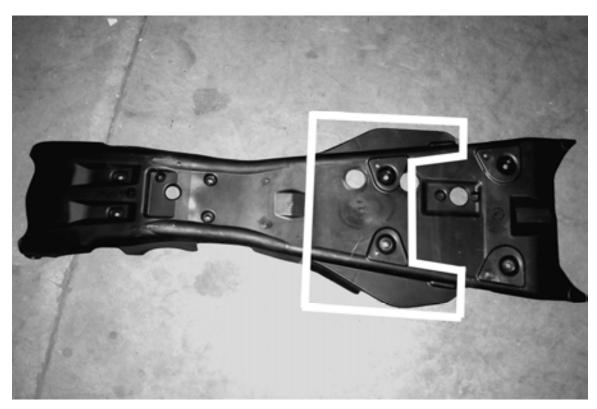
2. Install U-bolts into place over frame and over front footrest supports. (Square U-bolts over footrest supports may be hard to insert and will sit crooked until tightened fully)
