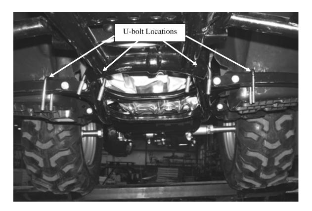
3. Install the blade mount loosely. Tighten the rear nuts on square U-bolt first to square the U-bolt up. The blade mount will trap tab created on rear section plastic skid plate between ATV and blade mount. Tighten remaining hardware.
